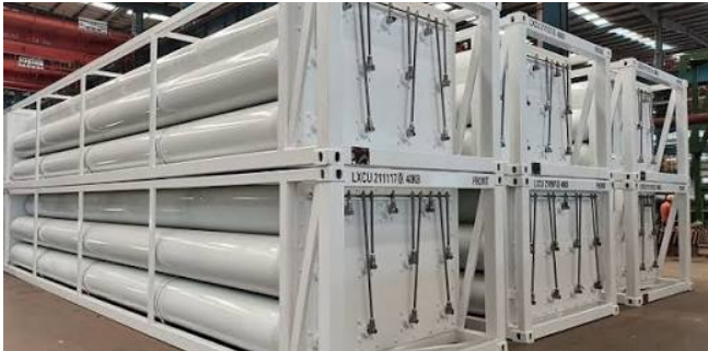
40 ft tube skids ready for despatch
